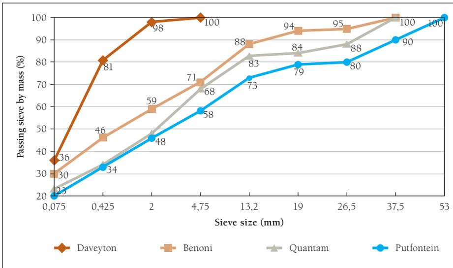
Figure 3 Grading curves for the material to be used
